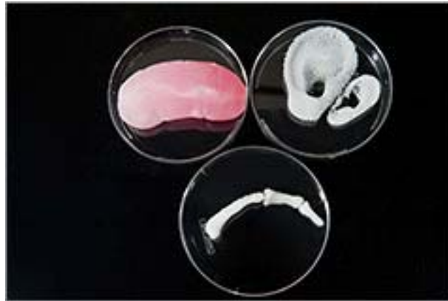
Figure 6. Images of 3-D-Printed Kidney, Ear, and Finger Bone (from CSC, 2012).
